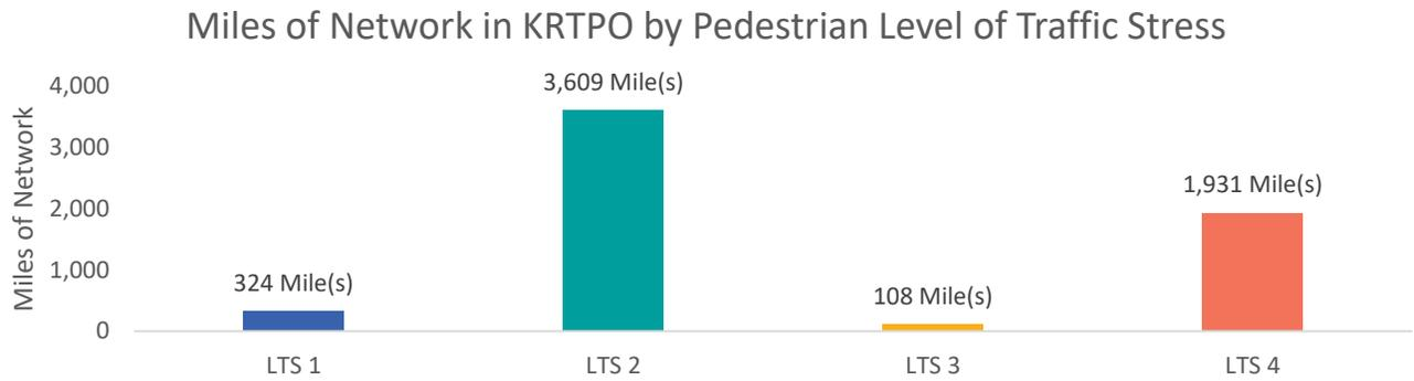
Figure 16. Miles of Network in KRTPO by PLTS
