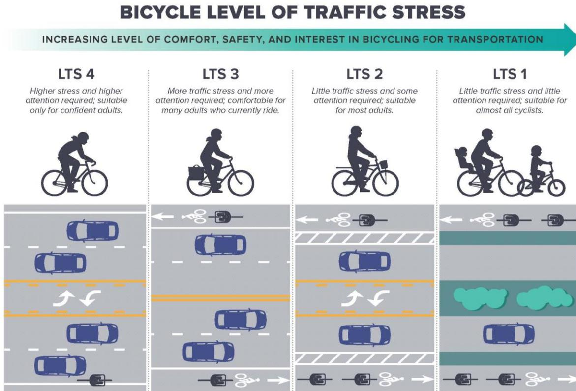
Figure 5. Bicycle Level of Traffic Stress Infographic
