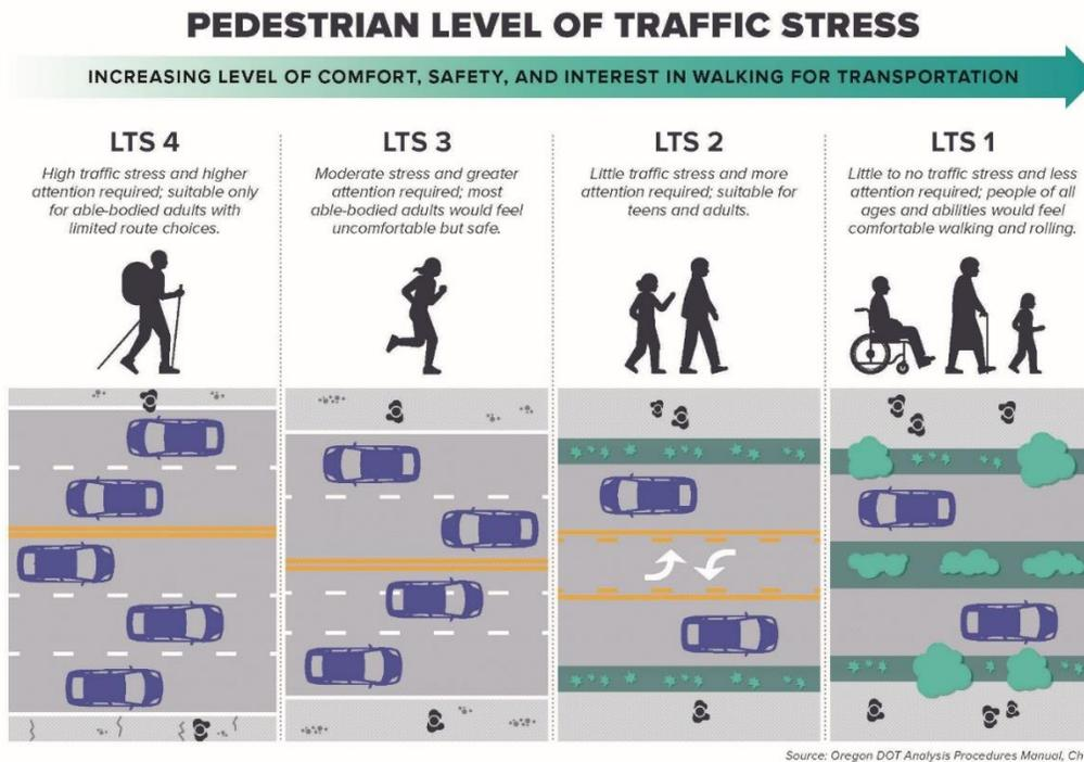
Figure 15. Pedestrian Level of Traffic Stress Infographic
