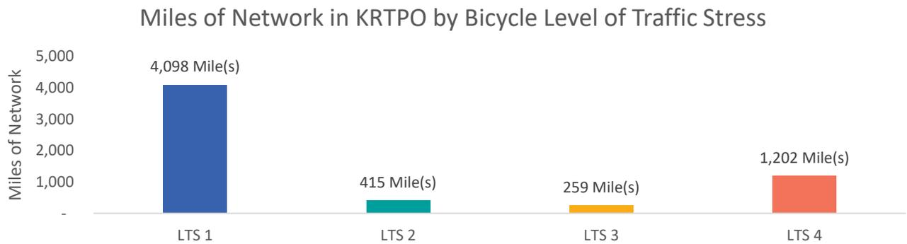
Figure 6. Miles of Network in KRTPO by BLTS
